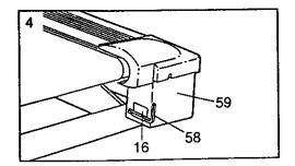
Using the 7/32" Allen Wrench (9), loosen the Handrail Bolt that is under the Console (6). Rotate the Console to the position shown.
